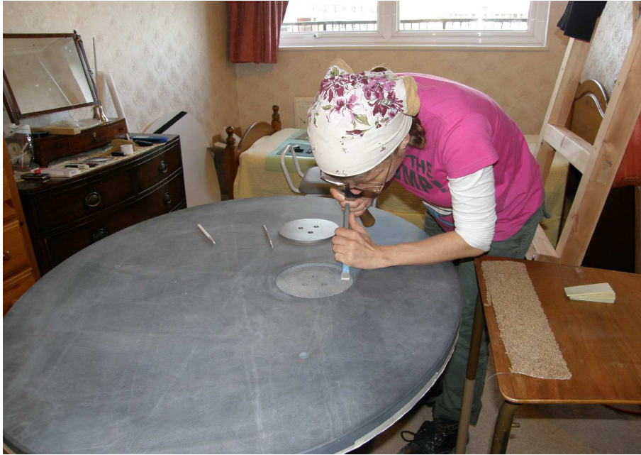
Fig. 43 — Annika Larsson cutting the Recess for the Base-Plate
